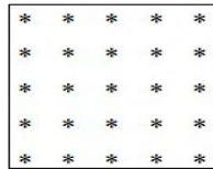
Figure 3.1: 5 \times 5 square structure element B
