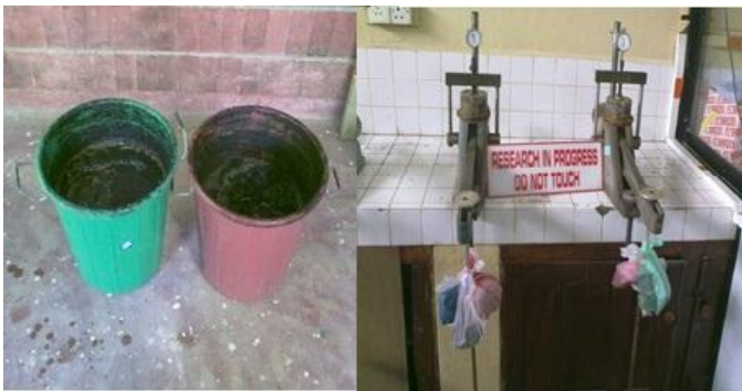
Fig 5 : Peat Sample as it's taken from the site & the Oedometer Testing in progress
