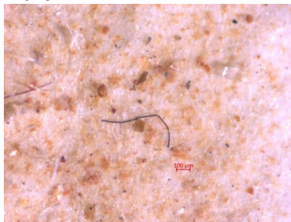
Fig. 6. Black Fiber Viewed Under Microscope
