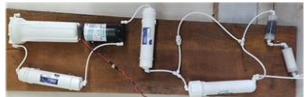
Fig. 7 Developed desalination unit
