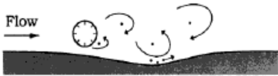
Figure 6: Sediment motion caused by vortex passing overhead.
