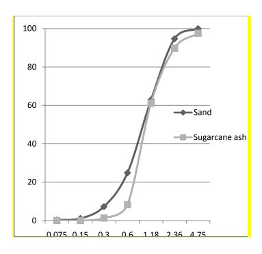
Fig 1. Comparison of sieve analysis between SCBA and sand
