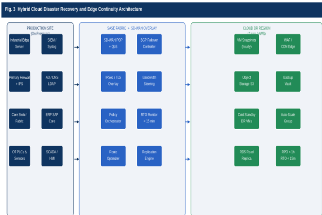
Fig. 3. Hybrid Cloud Disaster Recovery and Edge Continuity Architecture — illustrating production site components, SASE fabric SD-WAN overlay with RTO monitoring and replication engine, and cloud DR region with VM snapshots, object storage, and automated failover meeting RPO < 1 hour and RTO < 15 minutes targets.
