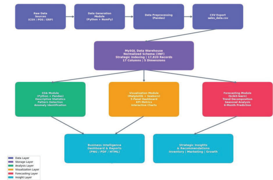
Fig. 1. System architecture of the sales analytics and forecasting platform.
