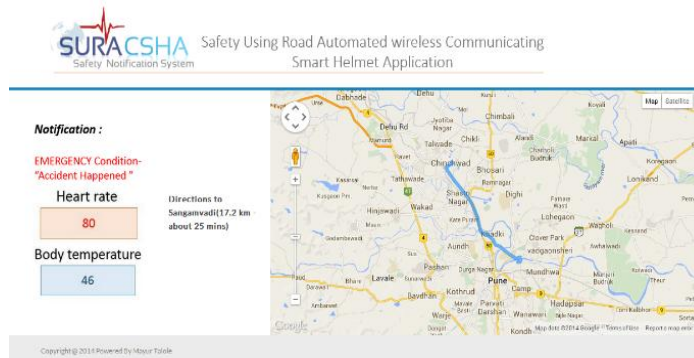
Figure 9: Image of the notification containing heart rate, body temperature and location of the person when the accident condition is detected
