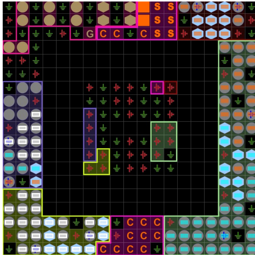
Figure 7.2.0.1: Standard cell layout showing routing tracks, power rails, decap, and filler cells
