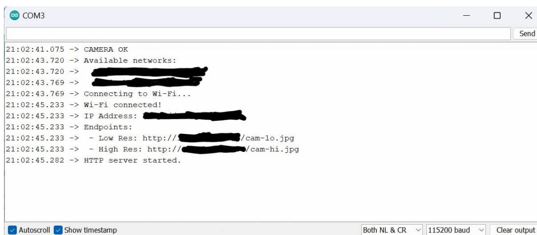
Figure D.1.0.2: Server Connection Establishment
