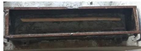
Fig.11: concrete beam with bamboo and steel
