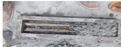
Fig.12: concrete beam with 2 bamboo and steel
