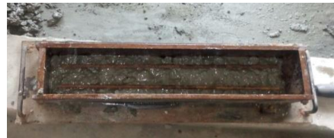
Fig.9: concrete beam with 2 steel
