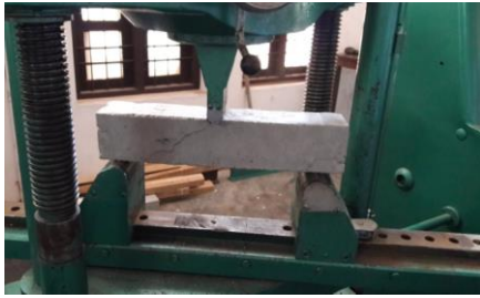
Fig.14: Testing of concrete beam with 2 bamboo and steel
