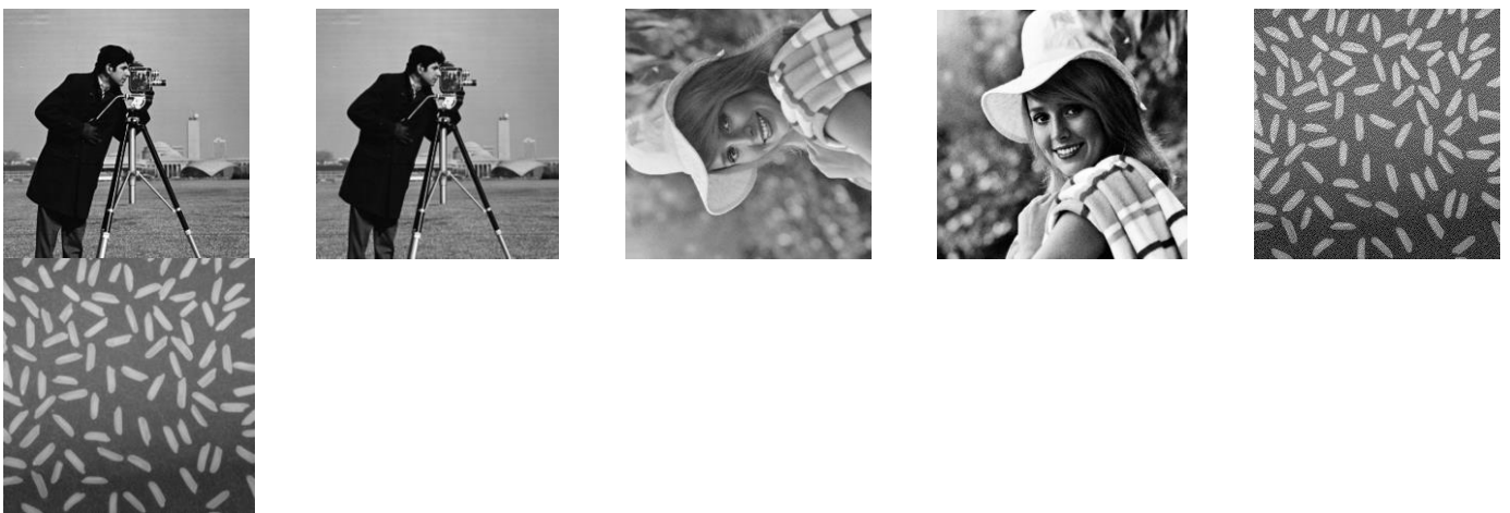
Fig.5. Watermarked images under different attacks (Sharpening, Gaussian Filter, Rotation, Histogram Equalization, Dithering, and Weiner Filtering)
