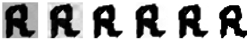
Fig.8. Extracted watermarks under different attacks (Gamma Correction, Median Filter, Pseudo Coloring, Cropping, Re-watermark, and Salt & Pepper Noise)
