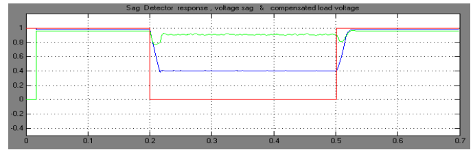
Fig. 8 Sag detector response, balanced voltage sag, compensated critical load voltage in pu in dqo system
