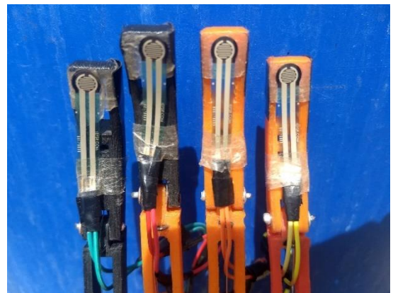
Figure 7 Placement of force sensors.
