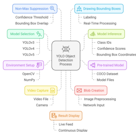
Fig. 3. YOLO Object Detection Process
