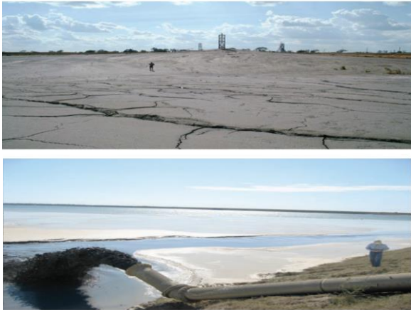
Fig 18. Dry and wet disposal comparison (Boger, 2013)
