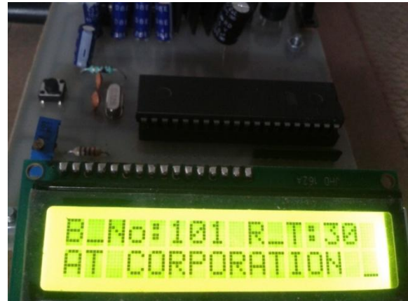
Fig. 15. Bus-Stop Module showing location of bus
