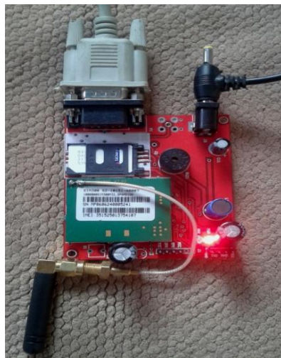
Fig. 8. GSM Modem at BASE-Station
