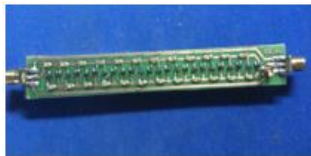
Fig. 10. 12-Stage Voltage Doubler
