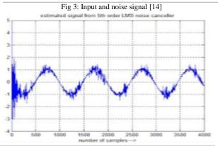
Fig 4: LMS filter output [14]
