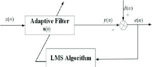
Fig 2: LMS adaptive filter algorithm [13]
