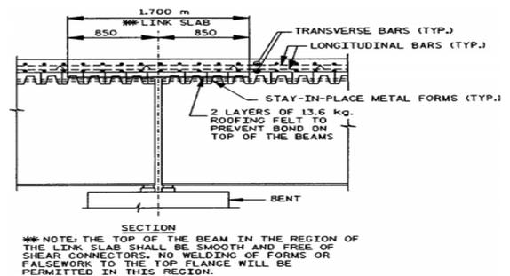
Figure 3: Link slab detail. Source [18].
