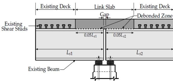
Figure 2: Debonded link slab configuration tested .Source [5].
