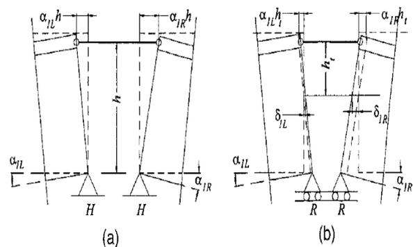
Figure 4: Force method for RHHR and HRRH Link Slab Bridge adopted from [19].
