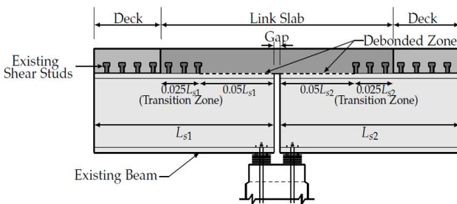
Figure 5: ECC link slab configuration proposed by [21].
