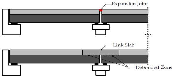
Figure 1: Deck joint replacement approach with link slabs
