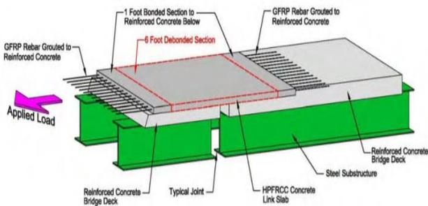
Figure.7: HPFRCC precast link slab tested by [36]
