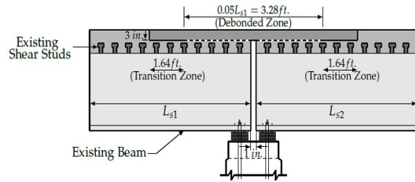
Figure.8. GFRP link slab detail
