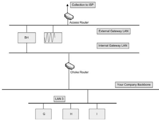
Figure 2: A sample packet filtering gateway
