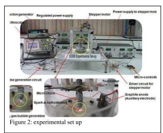
or pulsed modulator, Continuous electrolyte flow. The tool must be continuously dipped in the electrolyte. The current required is generally in the range of 5- 20 ampere and voltage is varied in the range of 25- 150 V. The schematic diagram of the process is shown in figure 1 and 2.
