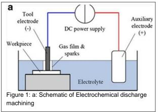
basic material removal done by spark erosion i.e. rough machining (stock removal) and electro-chemical affect – smoothens the surface of the work piece. The first work on electrode effect, anode or cathode effects
