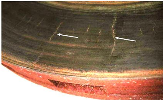
Fig.5 Thermal Cracking in Disc Brakes [11]
