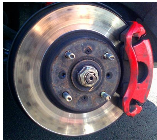
Fig. 4 Hotspot Generation in Disc Brakes [10].
