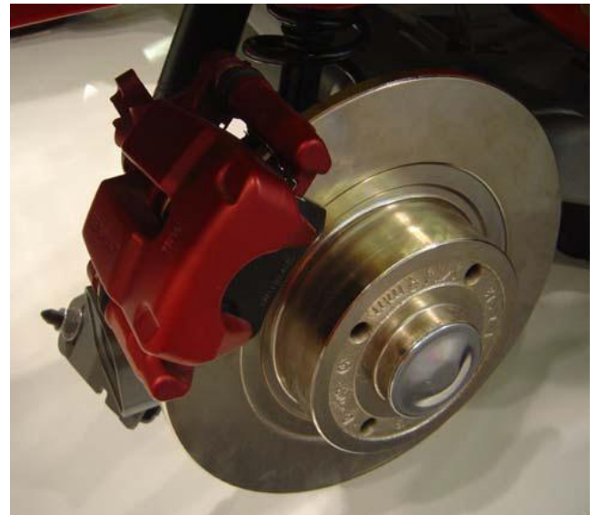
Fig. 2 Disk brake rotor, pad, and caliper assembly [2].
