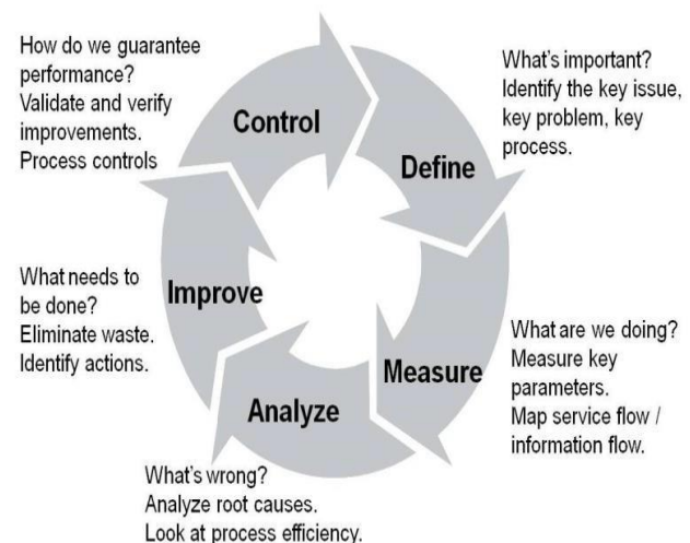
Figure 1: DMAIC Approach of Six Sigma Methodology
