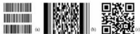
1.2 Evolution of barcodes: (a) multiple barcode layout, (b) stacked barcode layout, and (c) matrix barcode layout.
