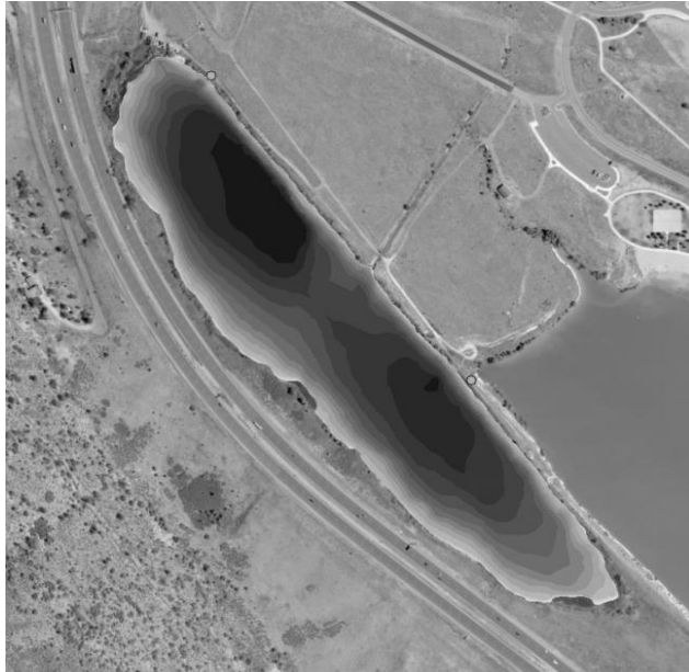
Fig.4. Depth analysis using Photo bathymetry
