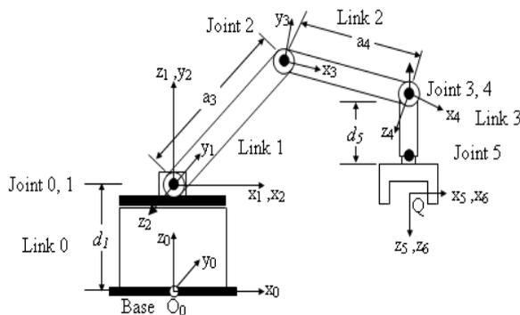
Fig 3.1 AL5B Robot Arm Frame Assignment
