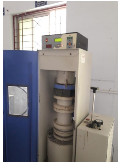
Fig 3 Experimental Setup for Compression test
