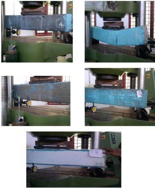
Fig 5 Testing of retrofitted beams
