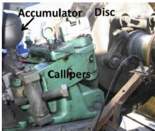
Fig.2. Photos of the hydraulic/accumulator system and calipers.
