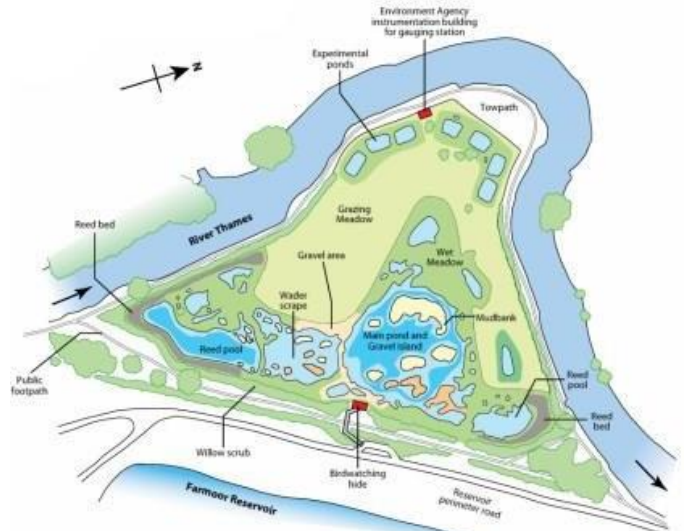
Figure 3 Diagram illustrating the creation of floodplain along the River Thames on Pink Hill Meadow in Oxfordshire (image from RRC Manual of Techniques)
