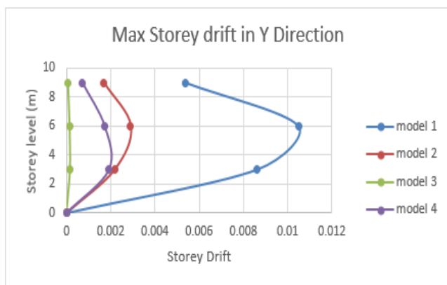
Figure 5.3 Maximum storey drifts in Case 1 in Y Direction
