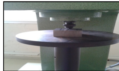
Figure7- Hardness Testing of Specimen
