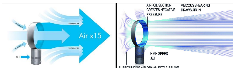
Fig -1: Air Multiplier Effect produced by a Bladeless Fan
