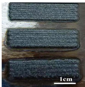
Fig. 2. Surface morphology of sedimentary layers at different laser power.
