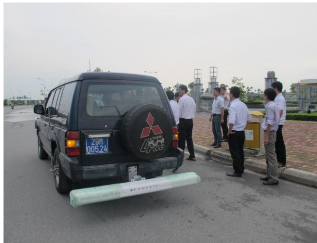
Figure 1. Pavement condition surveying car Hawkeye
