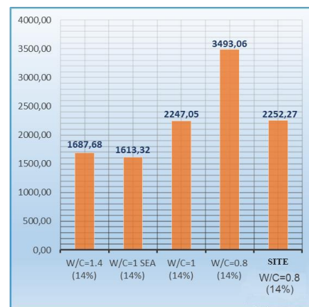
Fig. 6. Comparison of the value of q_u (kPa) between lab and field experiments
