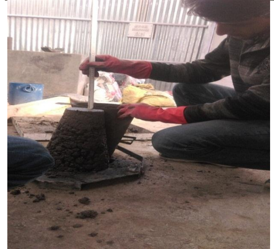
Fig. 9. and 10. Slump Test
