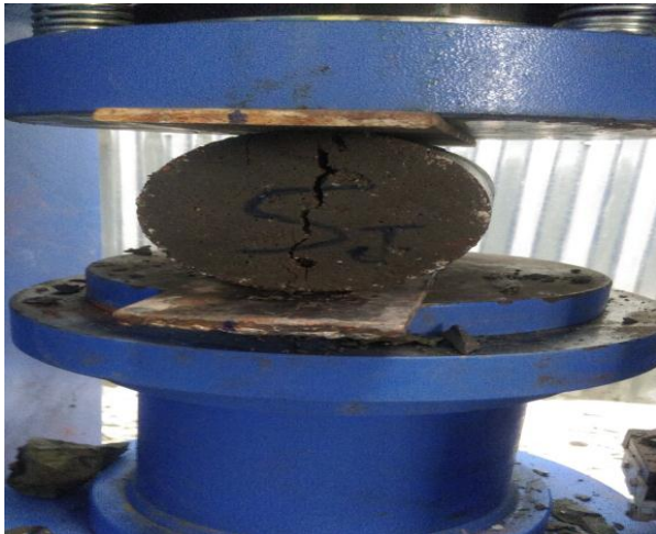
Fig. 17, 18, 19 and 20. Split Tensile Strength Test
