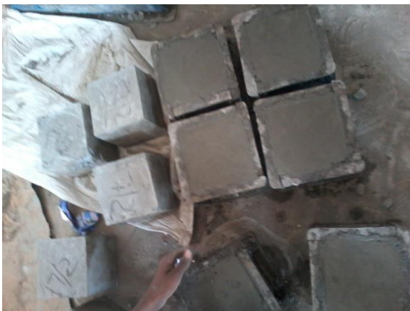
Figure 2 casting on cubes
