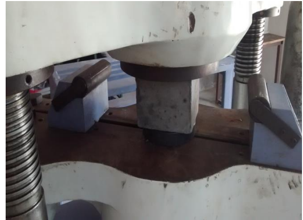
Figure 3 compressive strength test
