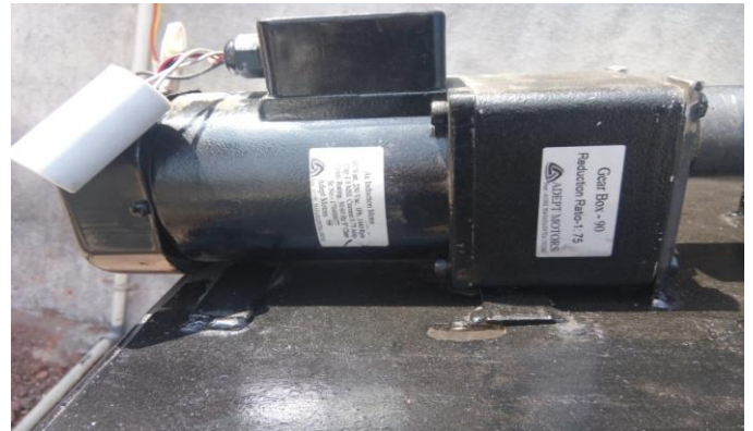
Fig.3.AC motor connected with gearbox
