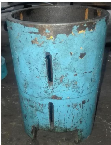
Fig 4.5 Liner guide way
