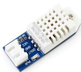
Fig. 2. Temperature and humidity sensing module (DHT11)
