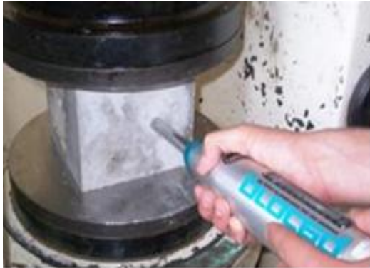
Figure 5.2: Rebound Hammer Testing
