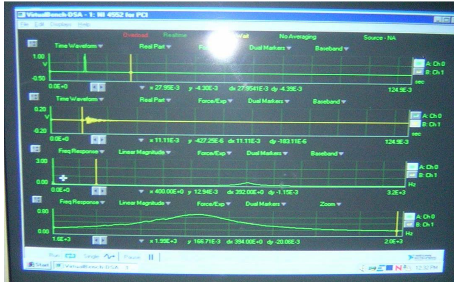
Fig.3-12: Results of transverse vibration of specimen shown on the monitor screen
