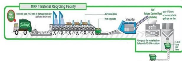
The above diagram shows the production of RDF from Municipal waste. The process involves collection of garbage and put it on material recycling conveyor where recyclable waste and non recyclable waste are getting separated. The non recyclable waste are collected by trommel and putting into
