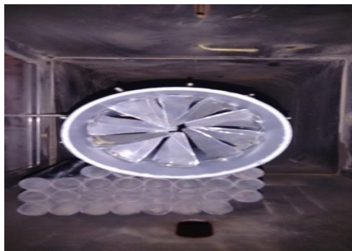
Fig 6.3 Guide vanes attached with test section area
