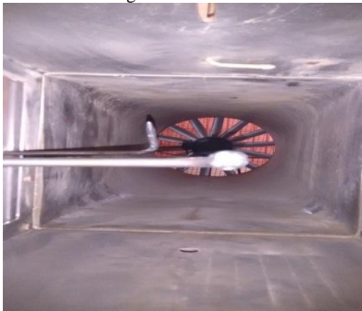
Fig 6.2 Five holes pitot tube
