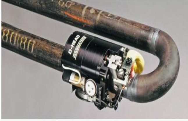
Fig 2.1 Orbital TIG Welding equipment
