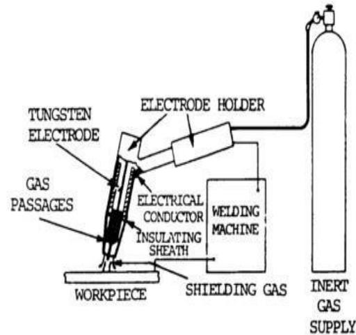
Fig 1.1 Schematic Diagram of TIG Welding
