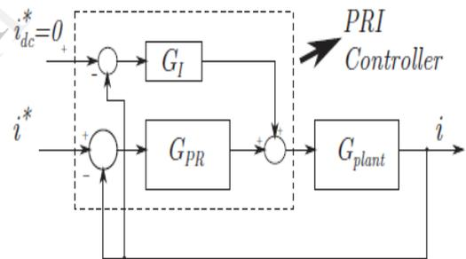
Fig.5: Block diagram of the fundamental current control with the PRI controller.
