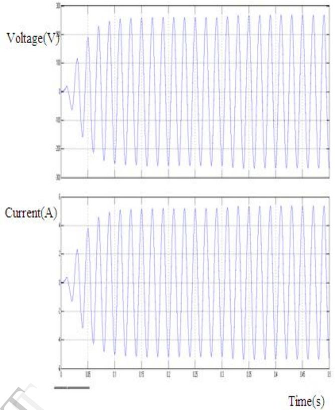
Fig.10. AC output voltage with the load connected to grid.
