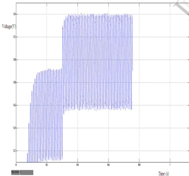
Fig 9. Boosted output DC voltage waveform.
