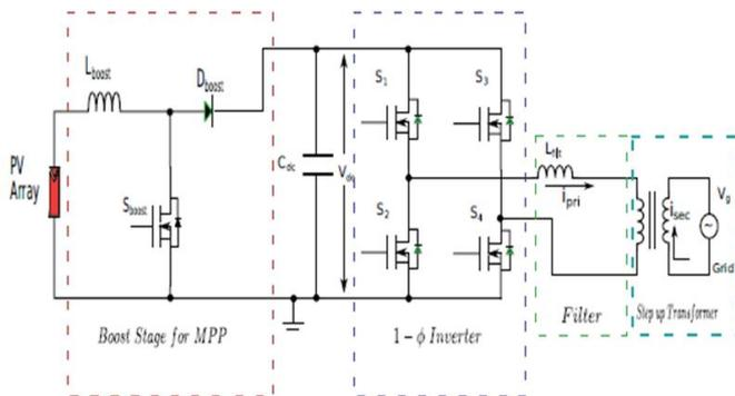
Fig. 2 Power Circuit Topology of single-phase PV System
