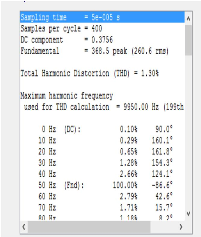
Fig. 11: FFT Analysis of output voltage.
