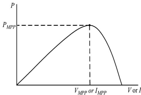
Fig. 3: P&O algorithm graphical representation
