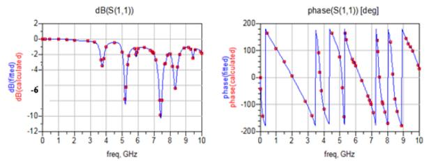
Fig.3(b).Bandwidth of Bowtie antenna
