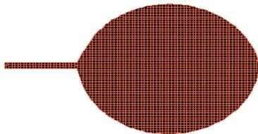
Fig. 5(a).Elliptical patch antenna
