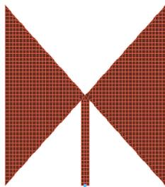
Fig. 3(a).Bowtie patch antenna
