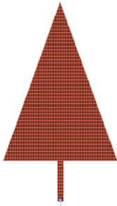
Fig. 4(a).Triangular patch antenna
