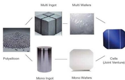
Fig.1. Manufacturing process of Solar Cell
