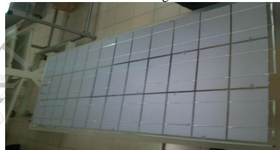
Fig.3. Stringing of Solar cells
